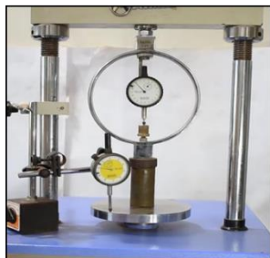
Fig 6: Set up for UCS test
