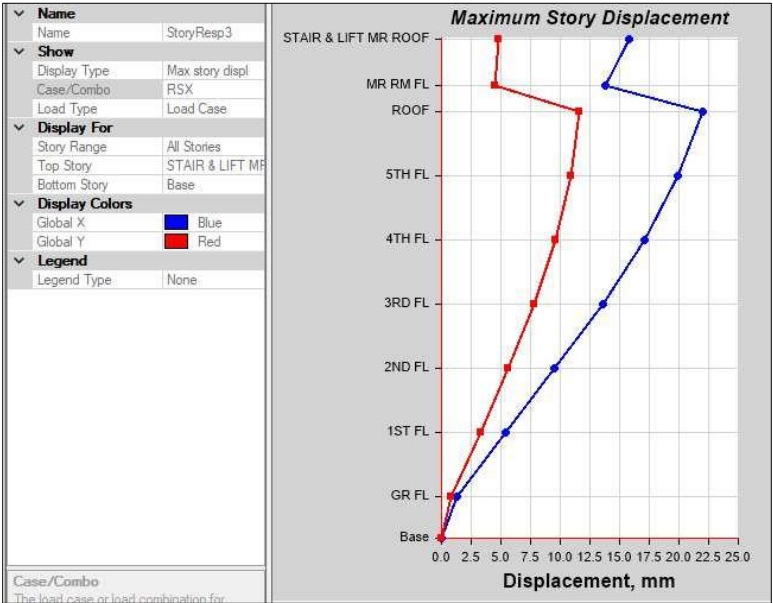
Fig. 15: Max. storey displacement due to RSY
