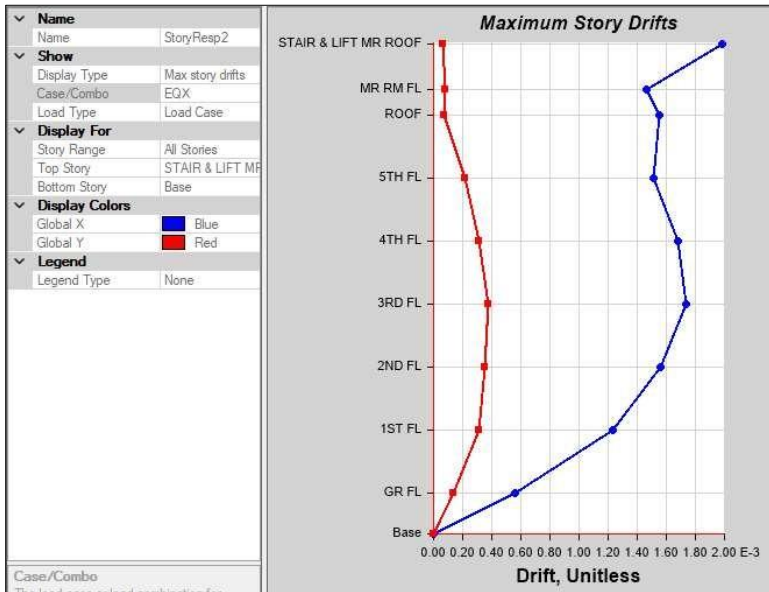
Fig 16: Max. Sorey drift due to EQX
