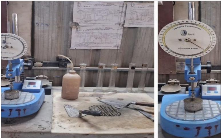
Fig 5: Testing of liquid limit by cone penetrometers apparatus
