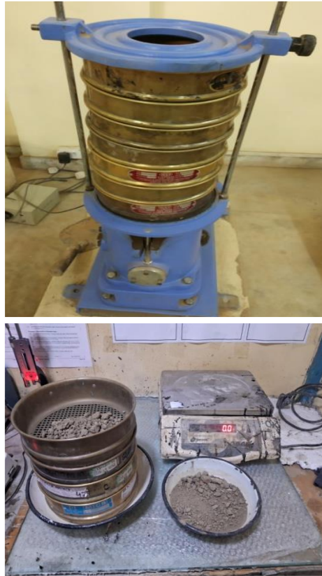
Fig 1: Instrument used in the study (a) Sieve Shaker (b) Set of Sieve
