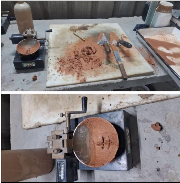
Fig 4: Testing of liquid limit by casagrande's apparatus
