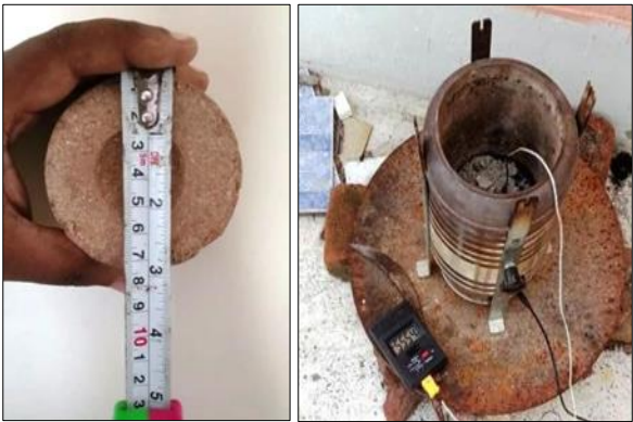
Fig 2: Sawdust briquettes burn in the commercial smokeless stove at a constant temperature of 500°C to 600°C
