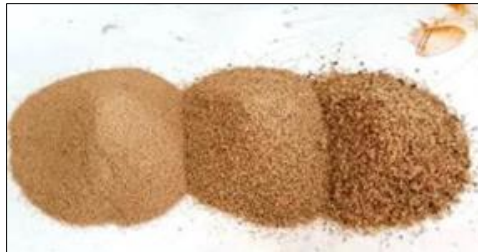
Fig 1: Standard Sand, >2mm-<1mm 33.3%, >1mm- <500micron 33.3% and >500micron-<90micron 33.3%
