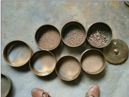
Fig 2.1: Sieve analysis of fine aggregates, Civil Engg. labs, GGV
