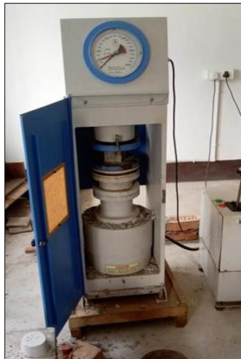
Fig 5: The compressive test as per IS 4031-6 (1988) at 28 days
