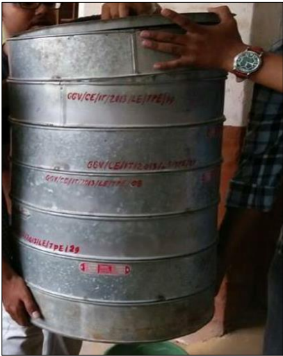
Fig 2.2: Sieve analysis of coarse aggregates, civil Engg. labs, GGV
