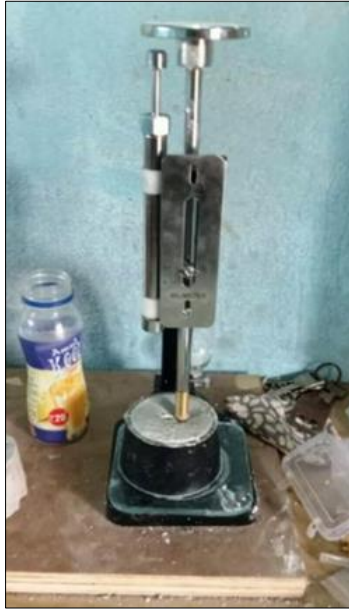
Fig 4: The standard consistency test following IS 4031-4 (1988)
