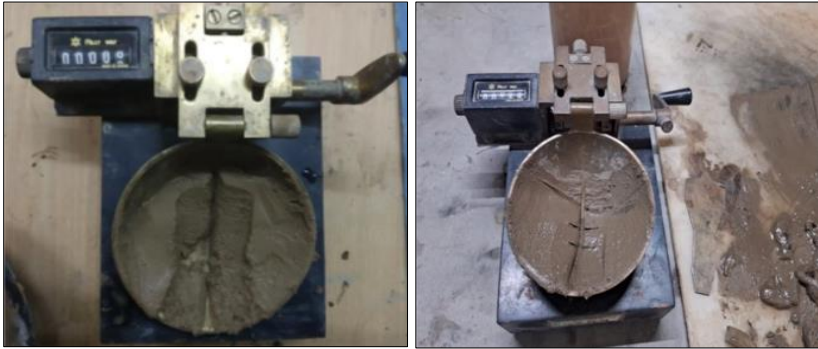
Fig 1: The device used in the study (a) Liquid Limit Device (b) Grooved Soil
